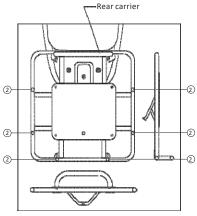
② Six "O" shape rubber washer installation positions.
